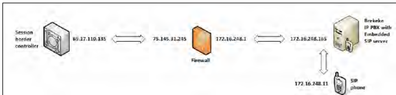
Figure 1.1 Brekeke PBX LAN topology, third-party firewall
