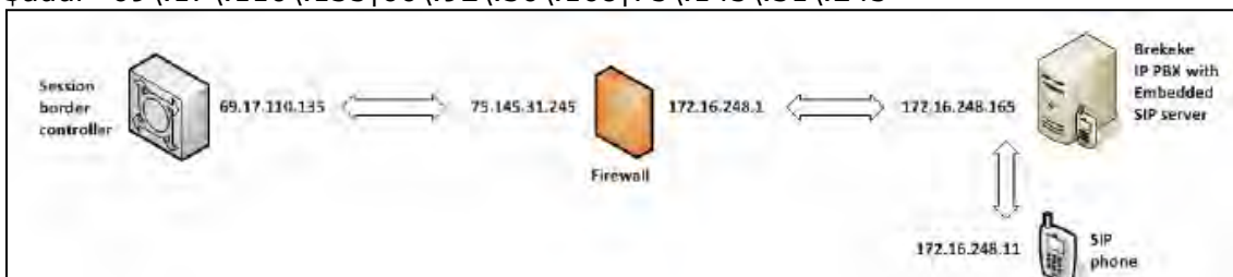
Figure 1.3.2 IP address scheme for SIP server Dial Plan
