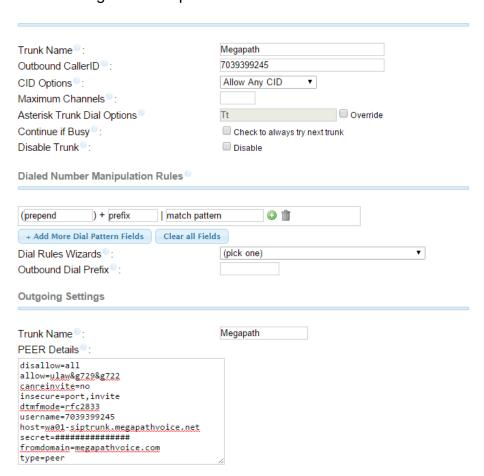
Figure: SIP trunk configuration with firewall
